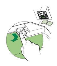
Position the new charcoal filter in the position marked and while holding the filter replace the fixing hooks as illustrated.
